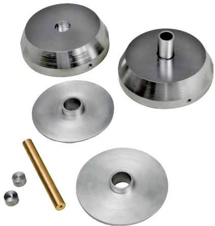
**Kit for ferrite powders measurements**
