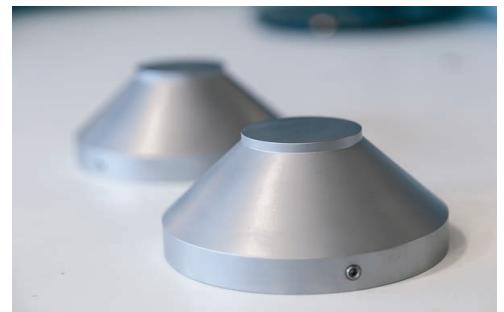
LPT Heating poles for high temperature measurements
