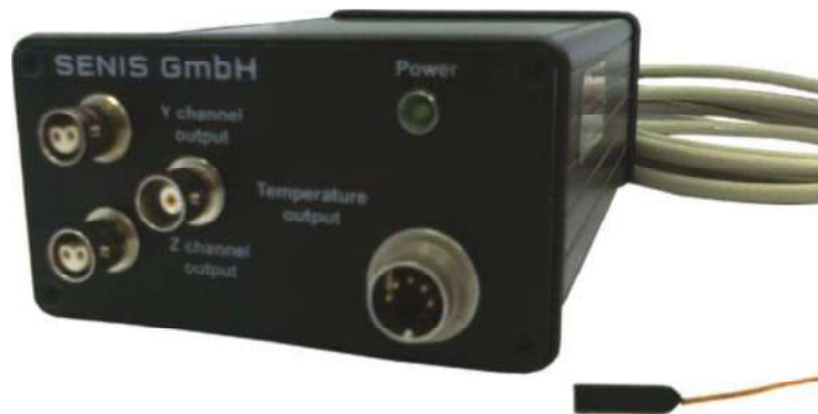
Figure 6. Front panel of the 1- and 2-channel Electronics module B
