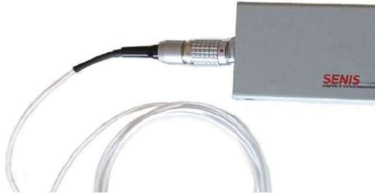
Figure 2. Photo of a 3-axis magnetic field transducer with a hybrid Hall Probe type "S". (The probe S can be fixed in a probe holder PHS-H, available at SENIS.)
