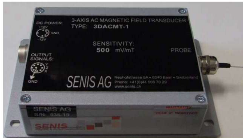
Figure 13: Photo of 3D AC Magnetic Field Transducer.
