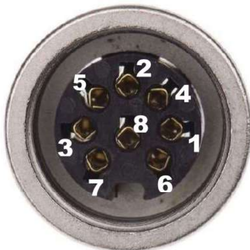
Figure 15: Output signal connector KVF 81 (matching with cable SV81 connector - pin out, front view)
