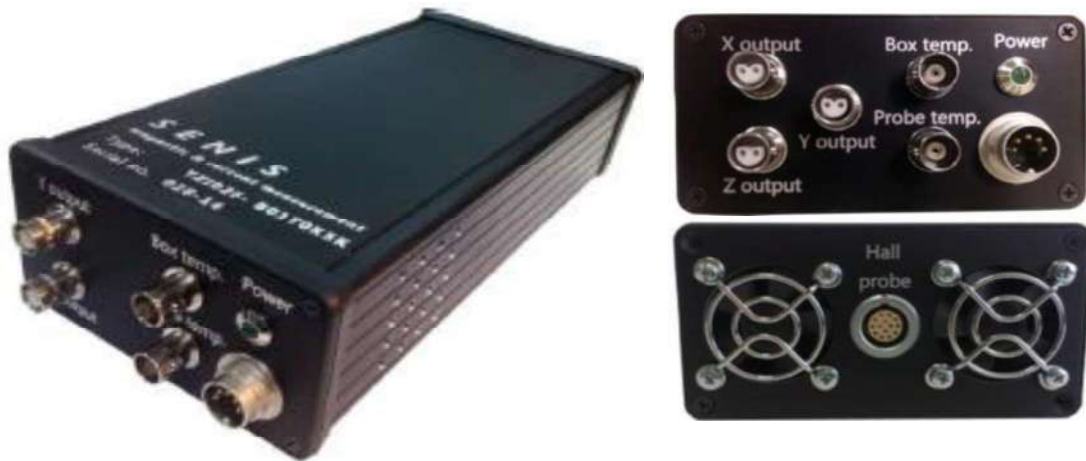
Figure 2. 3-axis magnetic field transducer I3A-03C02F-B02T0K5J
