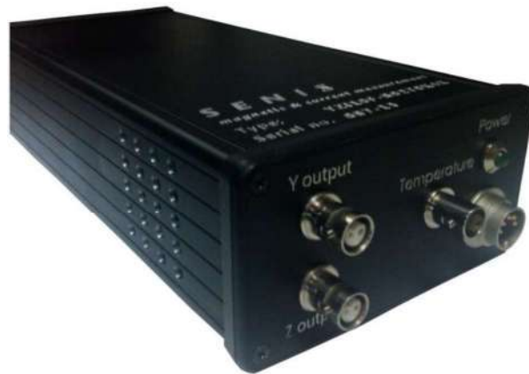
Figure 5. Electronic box (type B) of the I3A magnetic field transducer
