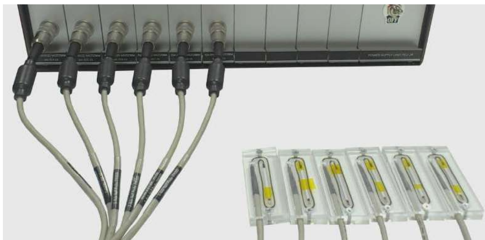
Figure 4. Single-axis Hall probes 0YK02D connected to the multi-probe system
