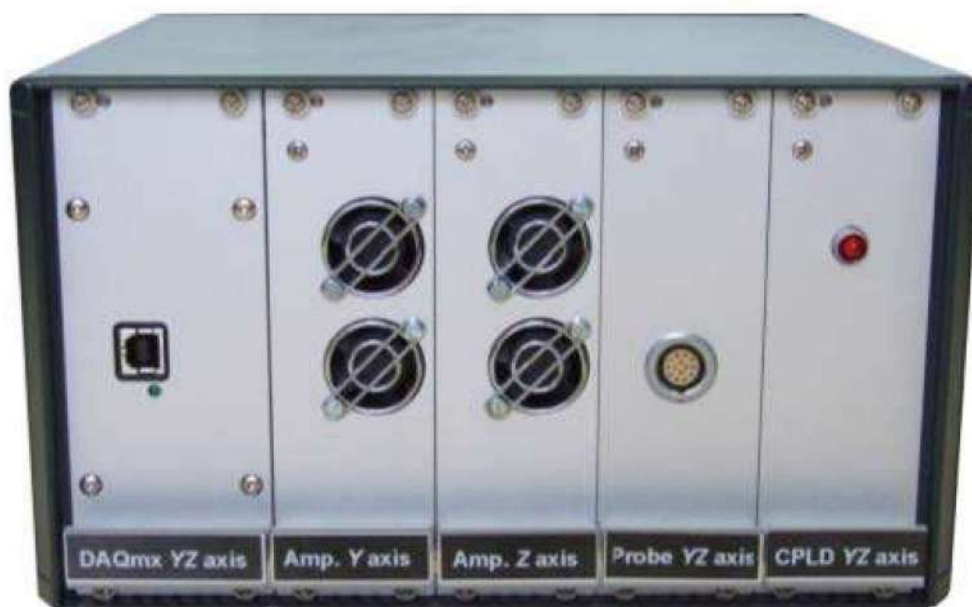
Figure 5: Electronic module with 16 bits ADS and sampling rate 400 kS/s. Dimensions are 235x133x255mm.
