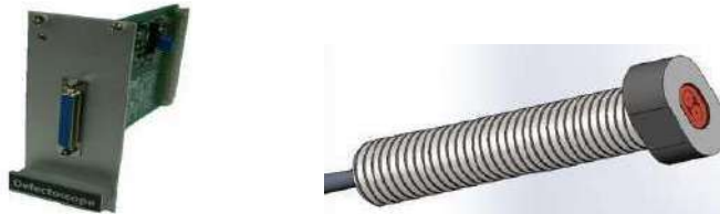
Fig. 6. Defectoscope electronic module and inductive probes mounted in the probe holder
